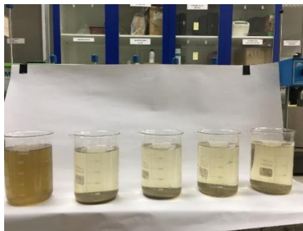
Figure 3. Abattoir wastewater after treatment (from left to right: dose of 0.5 g; 1.0 g; 1.5 g; 2.0 g and 2.5 g of moringa seeds powder biocoagulant)
