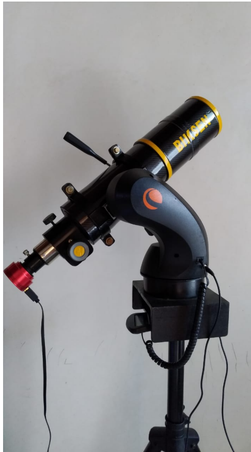
Figure 7: Handmade Refractor Telescope that has been connected to the ZWO ASI224MC astronomy camera and Celestron Alt-Azimuth mounting. 33
