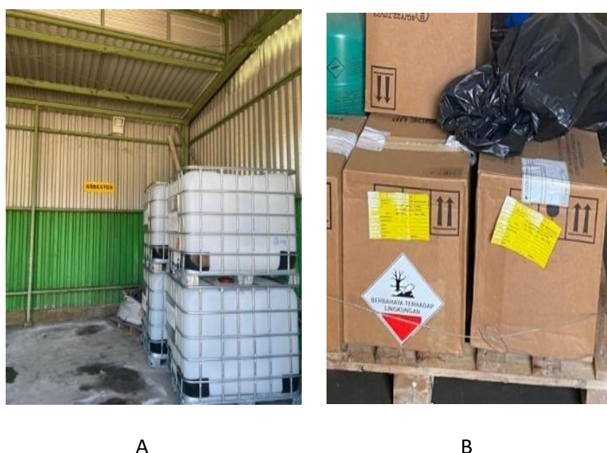
Figure 4: Symbol and Label Labeling on Hazardous Waste Packaging (A), No Hazardous Waste Symbol on the Wall and No 'EMPTY' Label on the Packaging (B)
