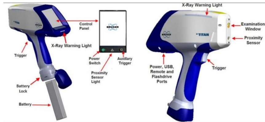
Figure 2. Main components of the Bruker S1 Titan 600 portable XRF analyzer
