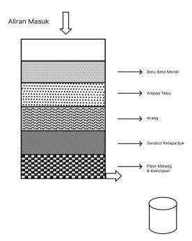
Gambar. 1. Unit media filtrasi multi layer
