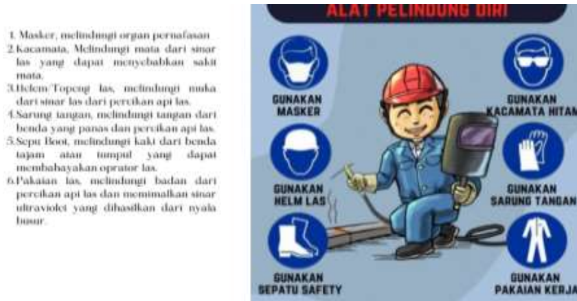
Figure 14. Personal protective equipment and its function
