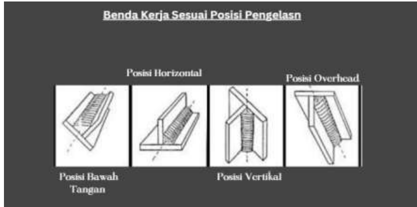
Figure 9. Position of the Workpiece Based on Welding Position
